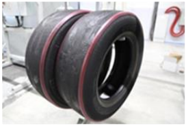
6) Cementing and cushion gum application
