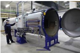
9) Intermediate product curing in the autoclave at a temperature of 117°C within 3 hours
